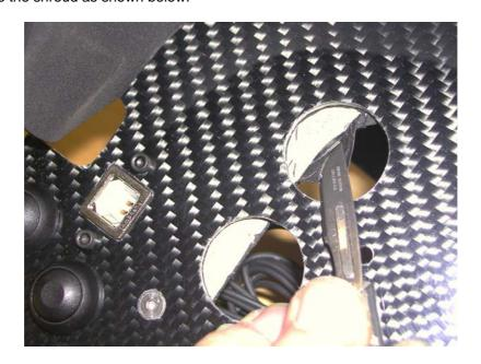
Using a scalpel or other suitable tool, remove the rubber covering in semicircles.
