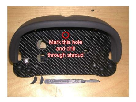
Step 7, Remove carbon panel and drill a 5 or 6mm hole through the shroud in previously marked position.
