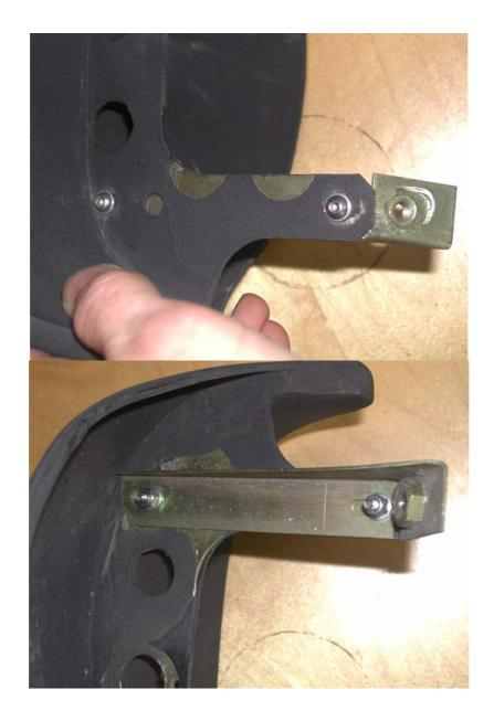
Step 9, Using a junior hacksaw cut a triangular wedge out of each semi circle. Use a rounded file or a hobby tool grinder to complete the semicircular cut outs.
