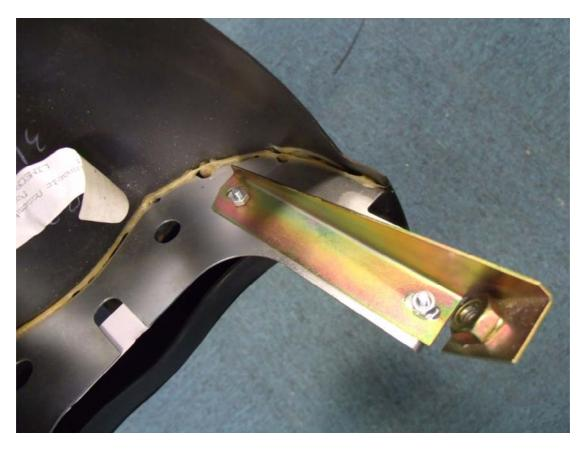
Ensure the bolt deepest inside the shroud is at the lower limit of the bracket's slot (with the bolts placed according to the template positions).
