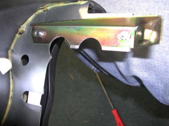
Unbolt the bracket and remove the paper template from the dashboard shroud.
