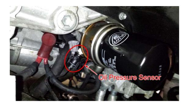
Remove the oil pressure switch and insert the oil pressure sensor. Check oil level once exchanged if much oil is lost.
