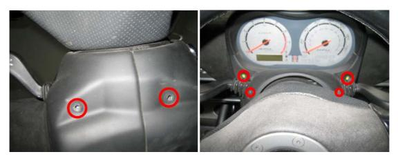
Remove steering column plastic covers by undoing the highlighted 6 screws and disconnecting the trip reset button from the lower section.
