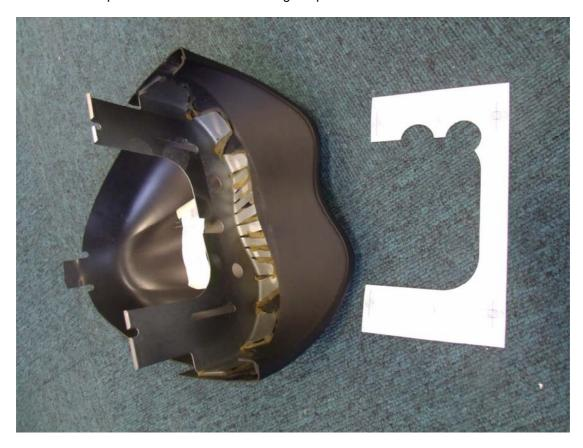
Using a temporary adhesive (e.g. Spray mount) stick this to the metal panel inside the shroud as shown:
