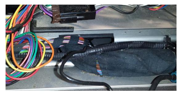
Once cable length needed is determined, cable tie where necessary between the centre console and the DASH2 PRO.  $\,$
