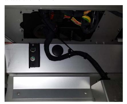
Thread the wire underneath the air vent tubes and insert the pins into the connector.
