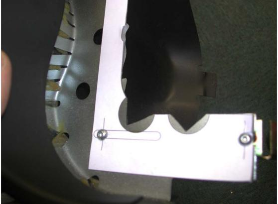
Using a file or a grinding tool, expand these cuts until they match the semi circular areas of the template.
