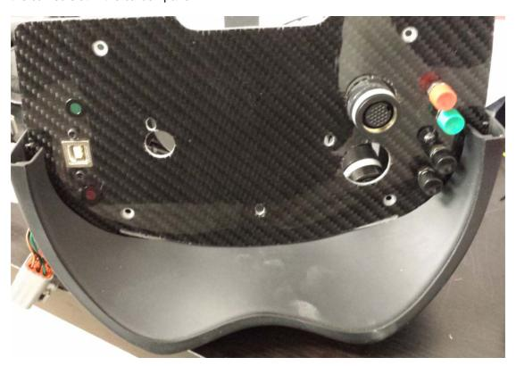
Press the carbon panel down firmly into the shroud, ensuring that the top of the carbon panel is touching the inside of the shroud. Included with the kit are 4 x 40mm long aluminium spacers. Squeeze two of these down, and position them for the deepest two panel mounting holes. (Note: these spacers are intended to be tight and with these two in position the panel should hold loosely in place).
