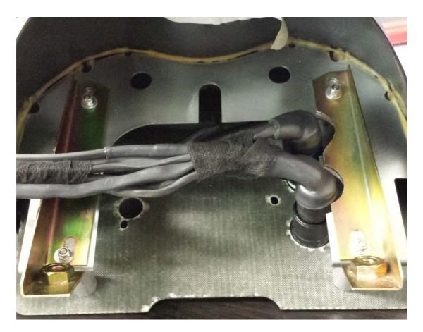
Bolt the DASH2 PRO to the front of the carbon panel, pressing the unit deep into the shroud so that the top of the unit (with the shift lights at the top) presses against the shroud section that slots through the carbon panel.
