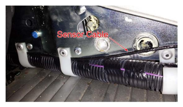
Now thread the cable through the centre console, following the existing cables/loom and cable tie where necessary.
