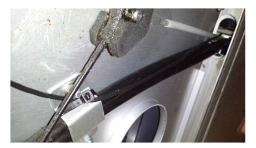
Unscrew and lift up the centre console (remove the handbrake cover by loosening the grubscrew) and pull through the cable.
