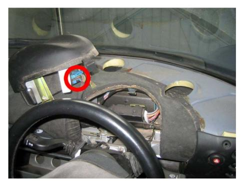
Disconnect the connectors from existing instruments.
