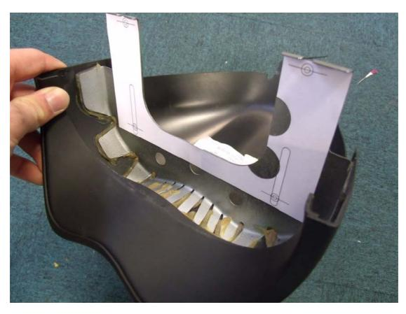
There are points marked where the bolts must go. Push some suitable bolts through at these points and bolt a bracket in place behind it as shown:
