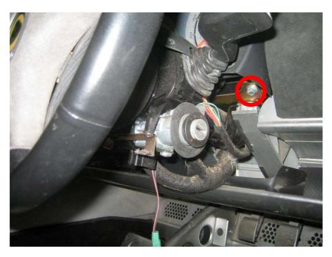
Unscrew 2 x 10mm hex head bolts and remove dashboard shroud.
