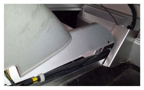
The original loom goes to behind the DASH2 PRO via a hole underneath the CD player. Remove the CD player and push the wire through the rubber seal.
