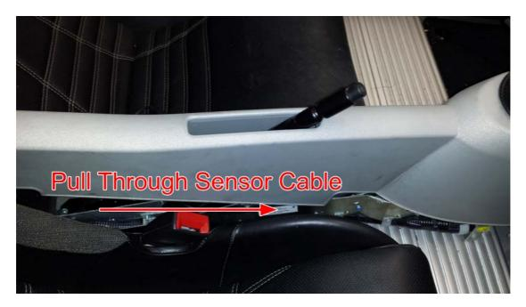
Thread the cable through the same holes and clips as the other wiring.
