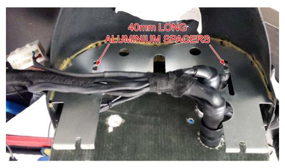
Feed through the M3 x 50 countersunk bolts. With the countersunk head on the panel, put the dashboard shroud mounting brackets behind (aligning the previously cut holes). Place a washer and nut over and loosely tighten.
