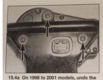
screws (arrowed) and remove the instruments
