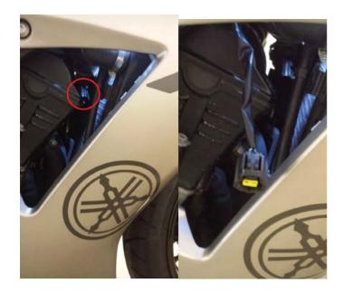
• Thread the inline connectors for the water temp sensor down to the water temp sensor
