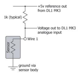
Once the sensor is connected to the DL1 CLUB with the pull up resistor then it can be calibrated in the normal way. For more information on this, please refer to this section. http://www.race-technology.com/wiki/index.php/HowDol/ConnectMyOwnSensor
