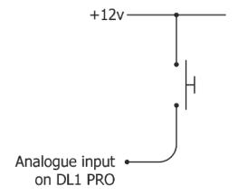
The "start/stop" button gives the driver the option of starting/stopping logging manually. Unlike the sensors that may be connected to the DL1 CLUB, the start/stop button has three connecting wires, and needs to be connected differently.
