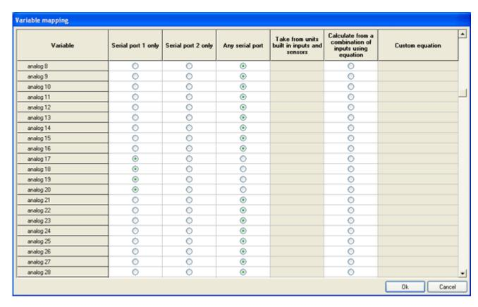
If you wish to take RPM data from the DASH2, scroll up and set the RPM to also come from the same serial port. If the option is greyed out for taking RPM data from the serial you will first need to disable the internal RPM sensor on the DL1 CLUB.
