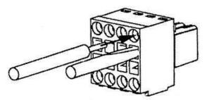
Now remove the screwdriver, leaving the wire to be gripped in place.
