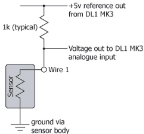
Once the sensor is connected to the DL1 CLUB with the pull up resistor then it can be calibrated in the normal way.
