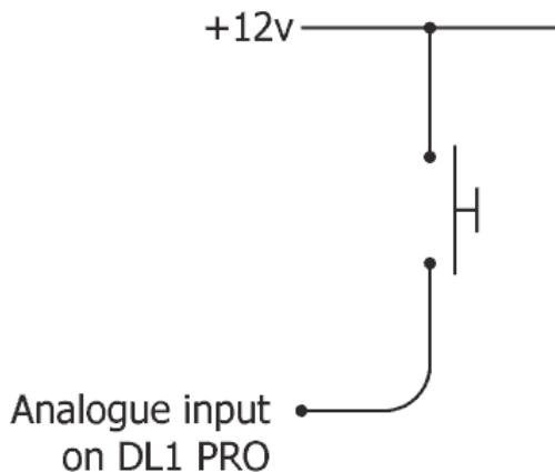
The "start/stop" button gives the driver the option of starting/stopping logging manually. Unlike the sensors that may be connected to the DL1 CLUB, the start/stop button has three connecting wires, and needs to be connected differently.
