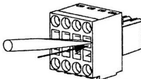
With the screwdriver still in place, insert the stripped and tinned end of the wire.
