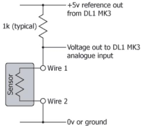
1 wire sensors are the same, but in this case the 2nd wire on the sensor is ground and made via the sensor body earthing to the engine casting etc.
