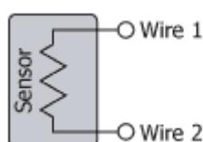
In this case we need to use a "pull up" resistor to convert the changing resistance to a changing voltage:
