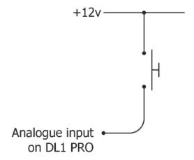
The "start/stop" button gives the driver the option of starting/stopping logging on the DL1 without having to press the button on the unit itself. Unlike the sensors that may be connected to the DL1, the start/stop button has three connecting wires, and needs to be connected differently.
