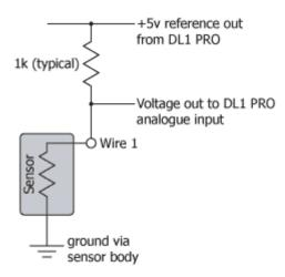
Once the sensor is connected to the DL1 PRO with the pull up resistor then it can be calibrated in the normal way. For more information on this, please refer to this section.
