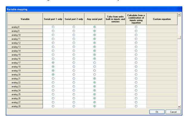
If you wish to take RPM data from the DASH2, scroll up and set the RPM to also come from the same serial port. If the option is greyed out for taking RPM data from the serial you will first need to disable the internal RPM sensor on the DL1 PRO.
